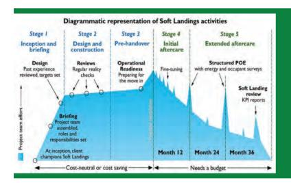
The vertical scale in this diagram is purely illustrative, hence the gradient of aftercare will be steeper or shallower depending on factors such as; how well was the protocol of Soft Landing followed from the initial stages, complexity of the building and the time scale within which the building will operate routinely (courtesy of BSRIA, Roderic Bunn)
